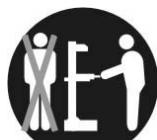
The log splitter must be used by one person alone.
