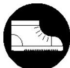
it is obligatory to wear safety footwear at all times to provide protection against the risk of logs accidentally falling on feet.
