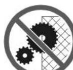
it is forbidden to remove or tamper with the protection devices and safety devices.
