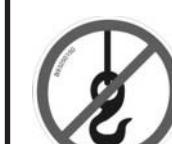
Do not use for connection: do not use the point shown in the picture to lift the machine
