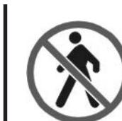
it is forbidden to stand in the range of action of the machine. apart from the operator, no other person or animal may be present within a radius of 5 metres from the machine.
