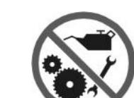
it is forbidden to carry out any maintenance work or renew parts on the machine when it is running.
